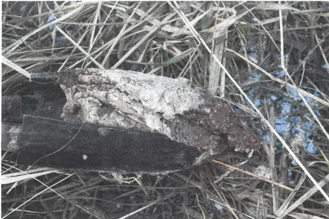
Figure No 1: The pit core with high content of energy gypsum (Photo M. Řehoř)
